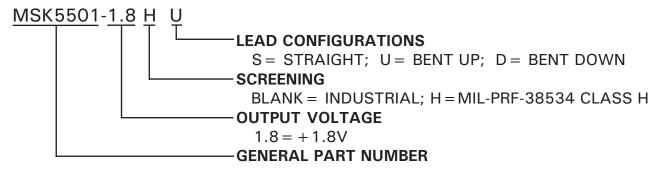
The above example is a +1.8V, Class H regulator with leads bent up.
